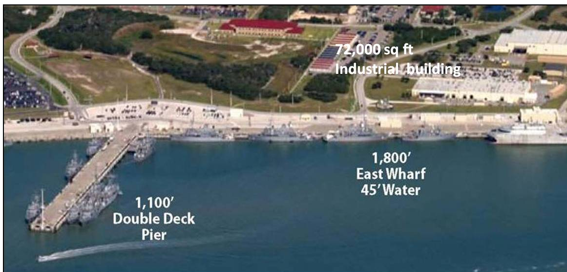
Figure 2. Capital-ship class 1,100-foot pier and the wharf area with its heavy load/unload capabilities.
